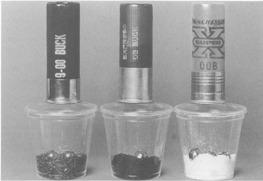
FIG. 1—Shot shells with pellets and buffer admixed in containers beneath each shell.
